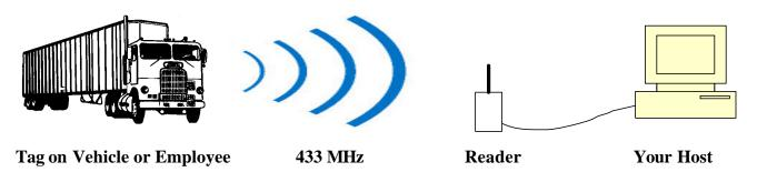
10' Range (Reader w/whip Antenna) - 50' to 300' with external Antenna
